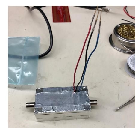
Feed the wires into a Male CONN housing (3pos) as shown on the right. Orientation of the pins is important, orient them as they are in the picture. You should here a snap/click once they are locked into position, however this is not always the case. The pins should be relatively uniform if they are positioned correctly. Give them a tug to ensure that they are secure in the housing
