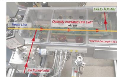
Figure 5. (Above) Image of SLIM drift tube ion mobility spectrometer with labels indicating location for optimal irradiation.
