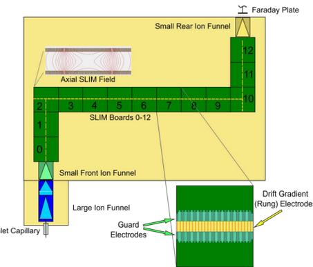
Figure 1. Simplified diagram of the SLIM ion mobility spectrometer design used to obtain the spectra presented within the results section.
