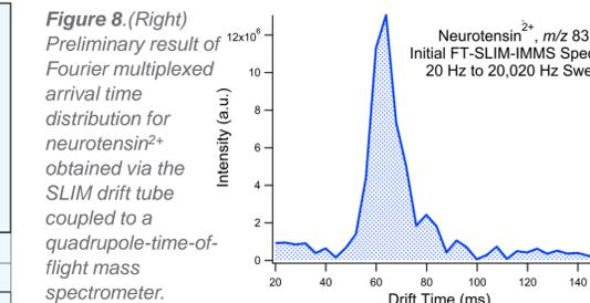
Figure 8. (Right) Preliminary result of Fourier multiplexed arrival time distribution for neurotensin<sup>2+</sup> obtained via the SLIM drift tube coupled to a quadrupole-time-of-flight mass spectrometer.
