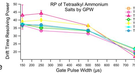
Figure 2. (Above) Using a mixture of seven homologous tetraalkyl ammonium salts (TXAs), the standalone SLIM drift tube's resolving power (RP) was assessed at four different gate pulse widths (150, 250, 500, and 750 μs). Resolving power is maximized using a 150 μs gate pulse width at ~37, and RP is maintained above ~30 up to a GPW of 500 μs.
