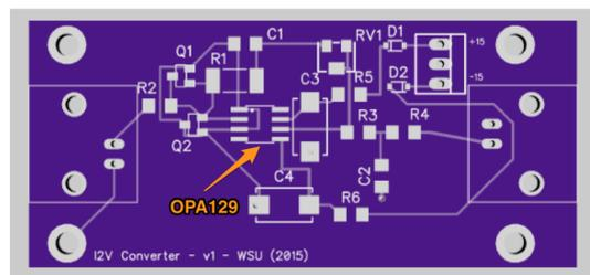
Figure 1. Circuit schematic for a current to voltage amplifier used for gains of  $10^8$  established through R1. Optimization of the amplifier circuit is required for higher gains. Diptrace and eagle files are located via github (<https://goo.gl/82c3Yo>)
