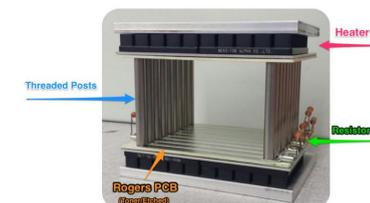
Figure 7. Prototype desolvation region with built-in gas heating. Electrode surfaces are made from Rogers 4350 PCB material and 0.1875 diameter stainless spacers. The dimensions are compatible with grounded insulation to minimize high voltage exposure.
