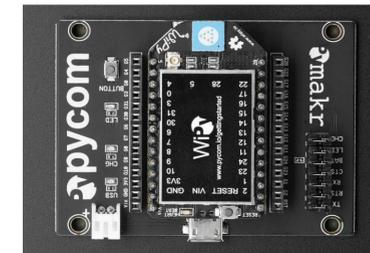
Figure 4. Wipy system mounted to an expansion board providing direct access to I/O pins and an onboard micro SD slot.
