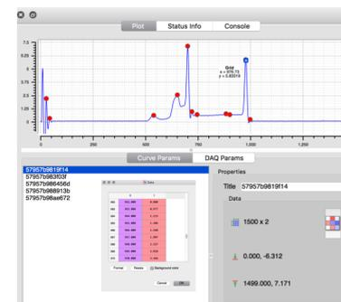
Figure 5. Cross platform GUI providing an interface to the local redis database. Additional features include data export, DAQ parameter uploading, and peak picking.
